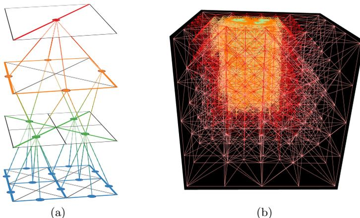
**Fig. 4.** (a) A *hierarchy of diamonds* (shown in 2D) is a rooted DAG whose nodes are the diamonds and whose arcs encode the the dependency relation among the diamonds. (b) Example variable-resolution tetrahedral mesh extracted from a hierarchy of diamonds. A tetrahedron’s color indicates its level of resolution.
