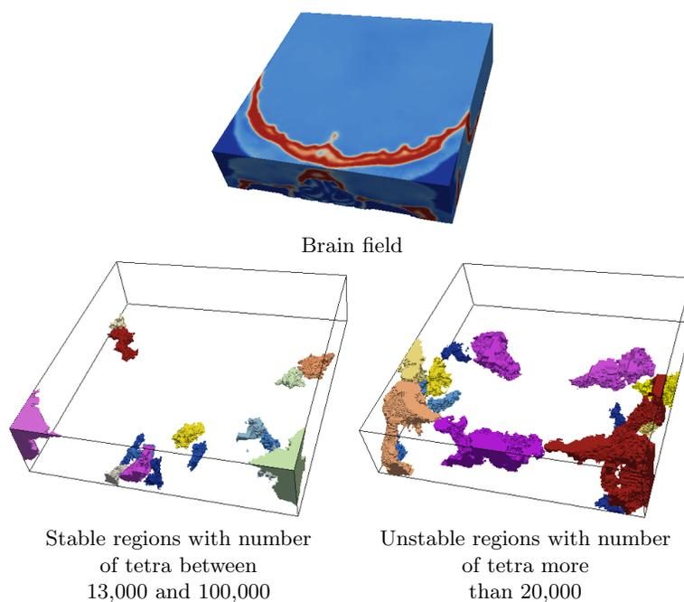
**Fig. 13.** Stable and unstable decompositions using a threshold to visualize distinct regions formed by a large number of tetrahedra.
